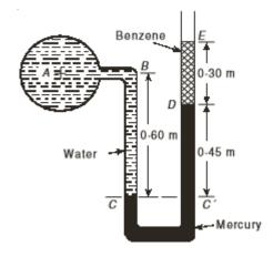
b) Briefly explain the principle employed in the 6 M manometers used for the measurement of pressure.
